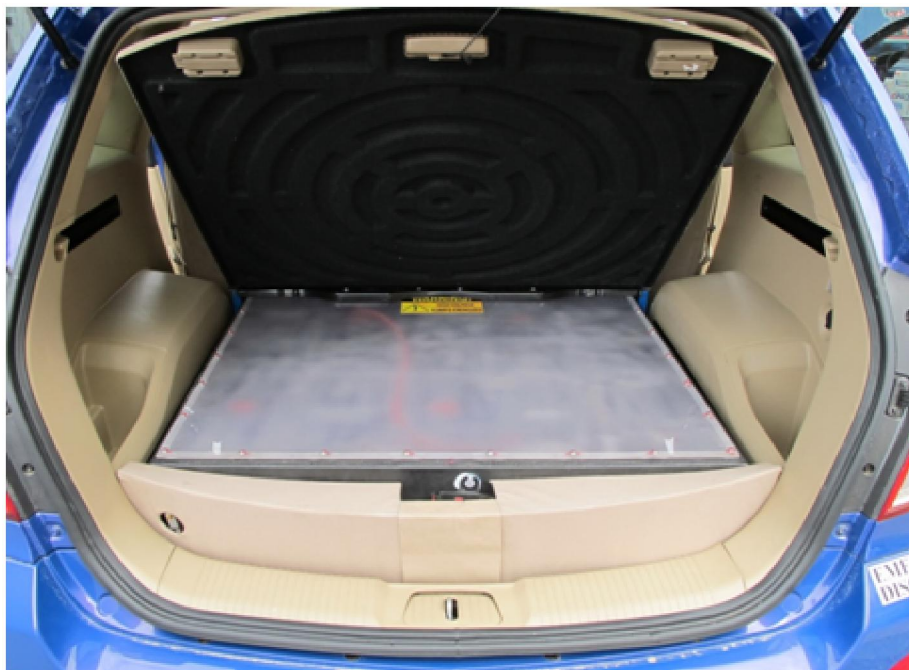
Figure 67 Close View of the Rear Cargo Area and Installation of the High Capacity Li-ion Batteries
